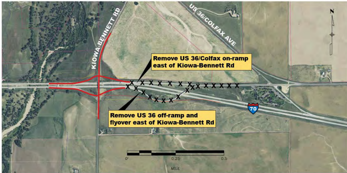
Figure 13: Kiowa-Bennett Road Interchange Configuration Options
